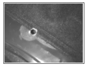
**STEP 4:** Place factory carpet back over hole. Locate the hole in the floor through the carpet and cut through the carpet to allow the mounting bolt to pass through the hole.
